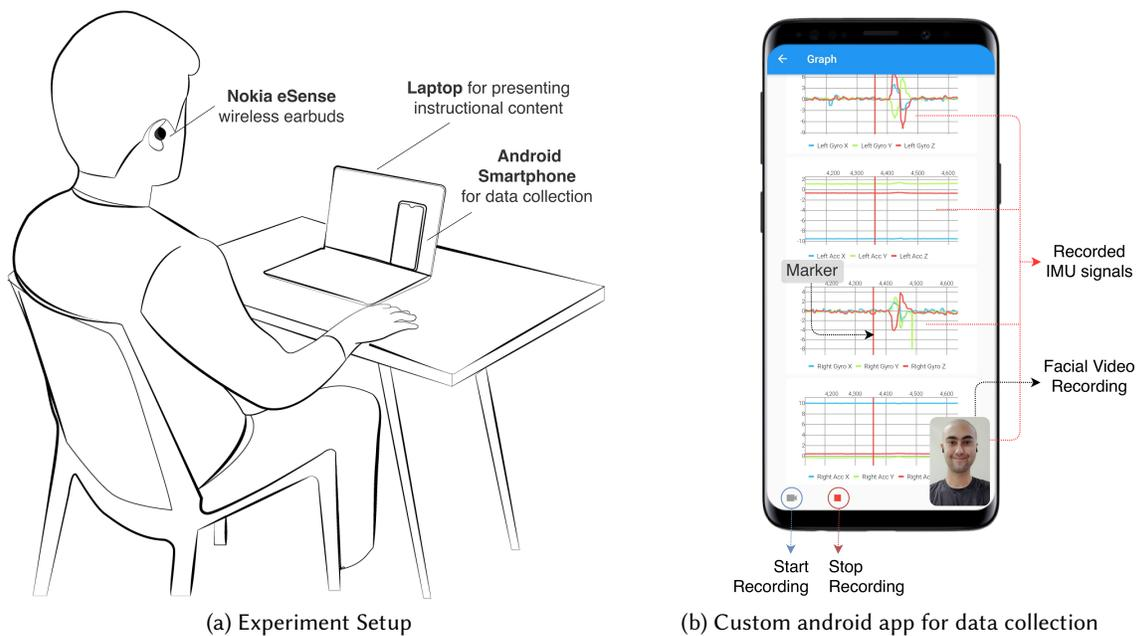
Fig. 5. Different components of the apparatus
