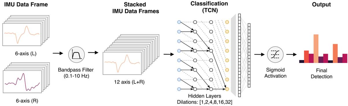
Fig. 4. ExpressEar’s processing and classification pipeline overview. Our temporal convolutional network (TCN) architecture comprises several convolutional units (four shown here) and one fully connected layer with sigmoid activation.
