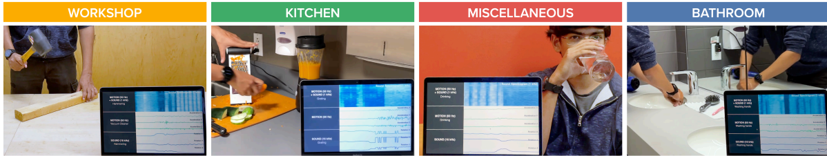
Fig. 5. Demo of SAMoSA running live in different contexts. Three models run concurrently for comparison, namely: the multimodal model (1 kHz audio + 50 Hz IMU), audio-only model (16 kHz audio) and the motion-only model (50 Hz IMU).
